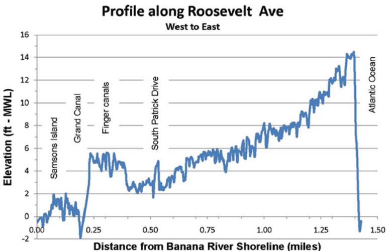
**Fig. 7** West to east topographic profile illustrating elevation of terrain along Roosevelt Ave (Figs. 3 and 4). As is typical of Atlantic Coast barrier islands, landscape elevation increases towards high-energy coastline (eastward). The elevated interval between South Patrick Drive and the Grand Canal reflects the presence of fill material acquired during dredging of the finger canals
